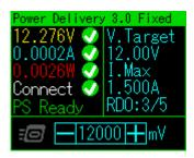
In fixed mode, the user adjust the voltage being triggered by scrolling the key to left or right.
