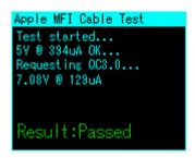
Connect the meter to a **QC3.0 supported** charger, and connect the MFI cable to the output port of the meter, the other side of the MFI cable should be left float.
