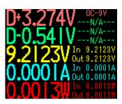
On the left side, from top to bottom, in big font are: D+ voltage, D- voltage, bus voltage, bus current, bus power. On the top-right side: Fast-charge protocols which are possibly running at the present.
