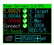
In PPS mode, the user adjust the voltage being triggered by scrolling the key to left or right (Each step is 20mV defined by protocol).
