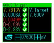
In QC3.0 mode, the user adjust the voltage being triggered by scrolling the key to left or right (200mV per step as the protocol defined.).
