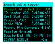
The top of the screen shows the CC pin which is in communication with the cable, followed by the raw data received from the cable.
