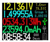
On the left side, from top to bottom are: current voltage, current, accumulated energy of the current accumulation group, accumulated capacity of the current accumulation group, accumulated time of the current accumulation group.
