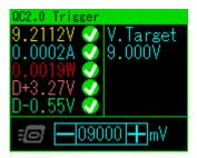
In QC2.0 mode, the user adjust the voltage being triggered by scrolling the key to left or right. On the left side, current meter readings are displayed to check if a trigger is successful.
